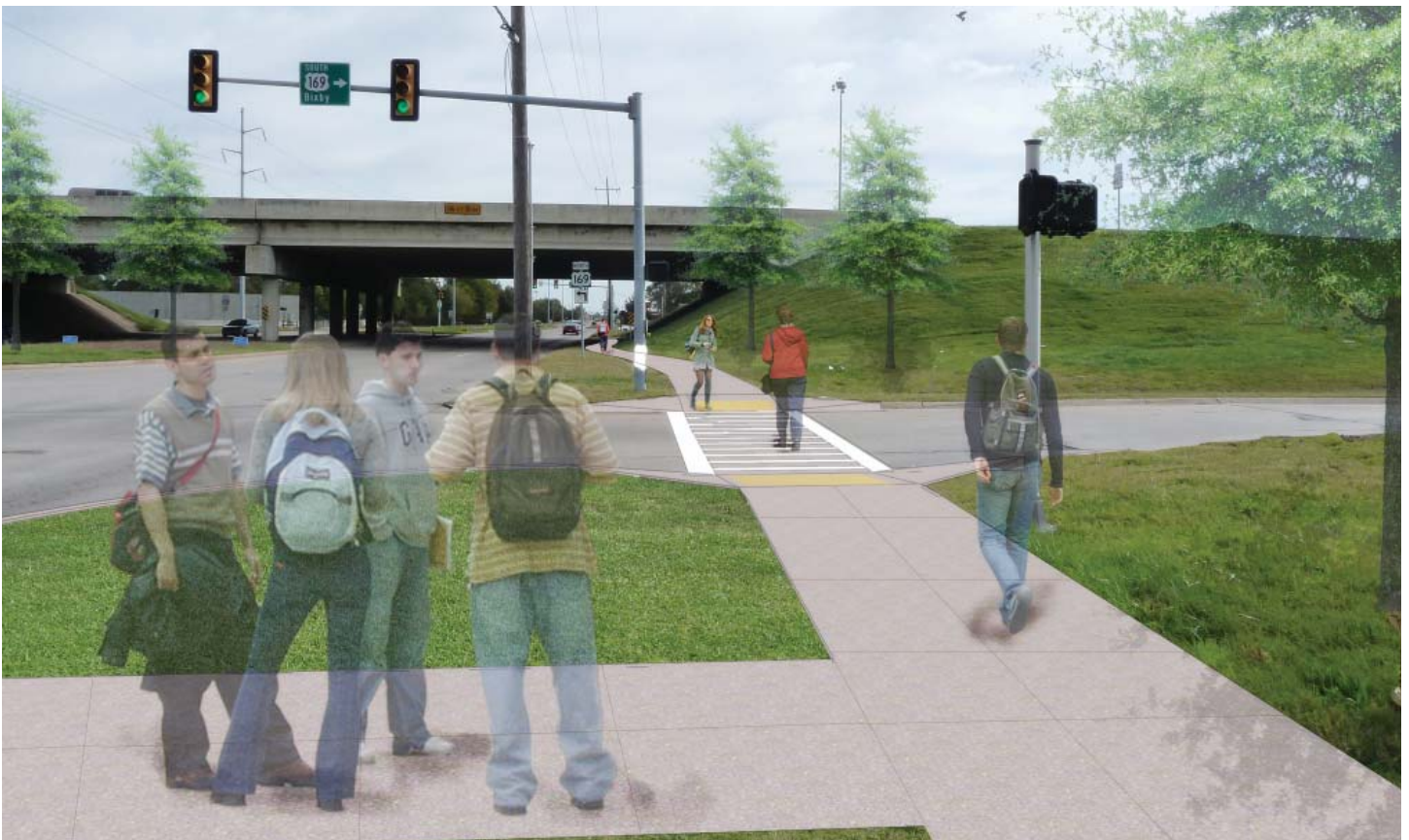
Conceptual photo-rendering of a high visibility crosswalk at the crossing of the Highway 169 on ramp
