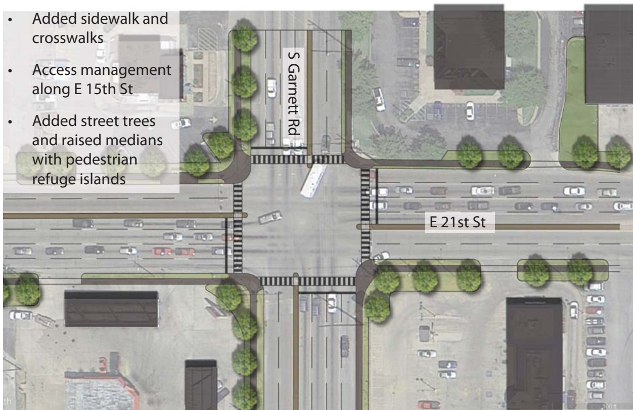
Conceptual plan of the proposed crossings, streetscape treatments, and sidewalk improvements at the intersection of E 21st Street and S Garnett Road
